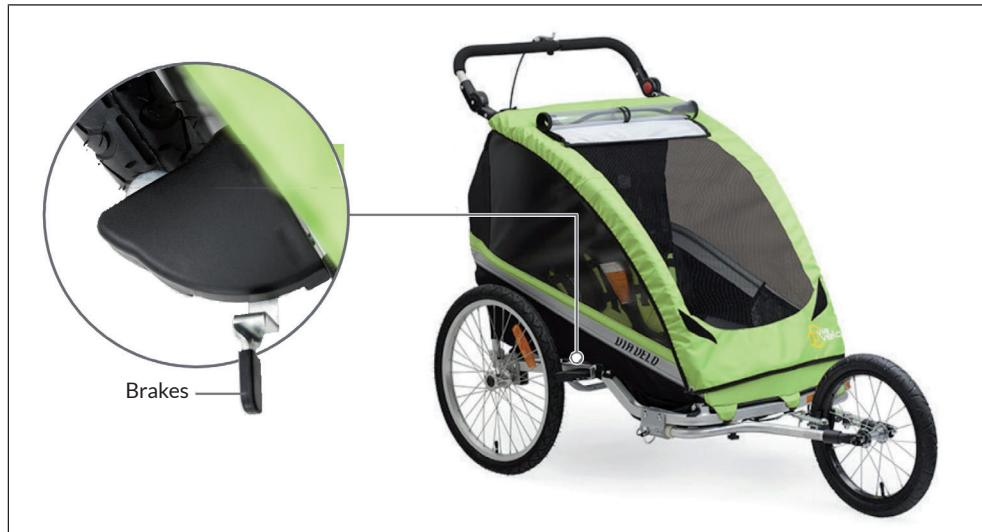
To lock the brake, move the brake lever outwards until it touches the tyre.
