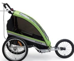
Press the red buttons on both sides and turn the handlebars to a comfortable position. Push the handlebars up or down to ensure that they are locked in position.
