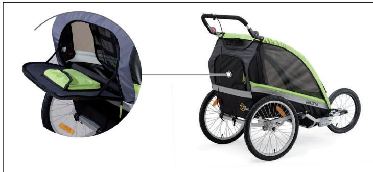
The trailer has a storage space. This is not intended for objects weighing more than 4.5 kg (10 lbs). To access the rear storage space, open the zipper on the back of the trailer.
