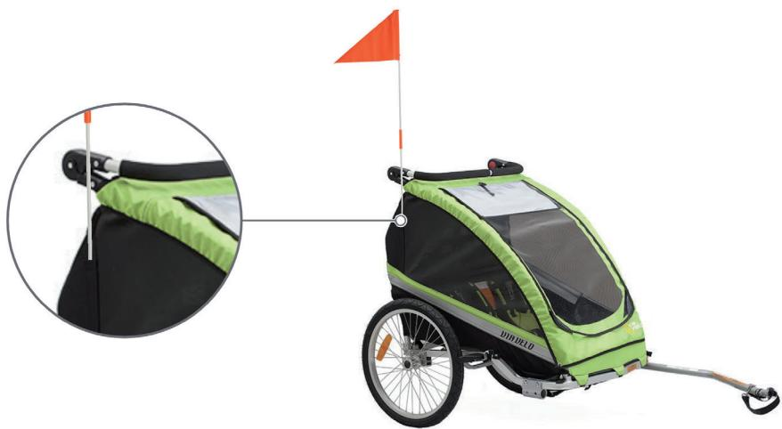
Insert the end of the safety flag into the small sleeve on the right side of the trailer.
