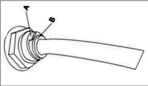
First remove the blue ring (A) and then press the white ring (B) on the outside. Remove the filling water pipe last.
