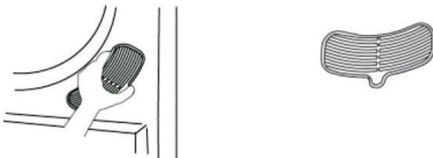
Clean the air inlet filter once a month. Remove the filter by holding the lower and upper ends of the frame and pulling it out. Clean the inlet filter with a soft brush. Then replace the filter in the frame and secure the frame.
