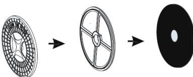
When you have cleaned the filters, replace them in reverse order. Make sure that the filters are firmly seated.
