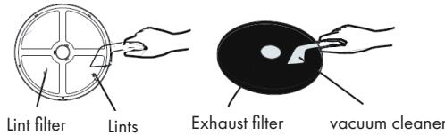
Separate the filters. Clean the filter cover, lint filter and exhaust filter with a soft brush or vacuum cleaner. Be careful not to damage the filters.
