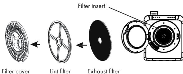
Remove the filter insert from the rear of the interior. The filter insert consists of 3 filters.
