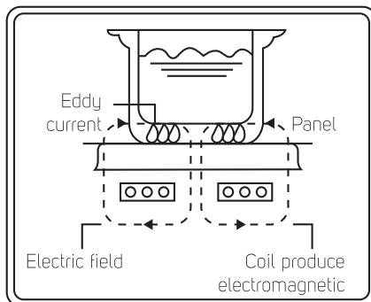
When the power connection is ON, the electric current will produce magnetic field in the induction coil, which is embedded in the machine. As soon as the magnetic force lines in the magnetic field touch the alloy steel pot/boiler, it will produce the heating effect, which would lead to the heating of the food in the pot.
