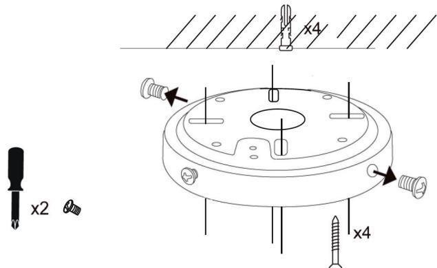
Fasten the ceiling plate to the ceiling with 4 dowels and screws.
