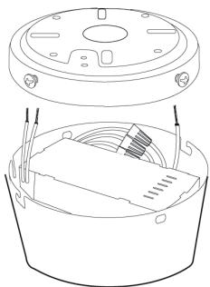
Insert the receiver and wires into the top cap.
