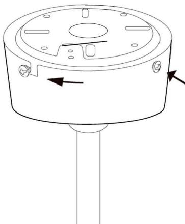
Fasten the upper cap and the ceiling plate with 4 screws.
