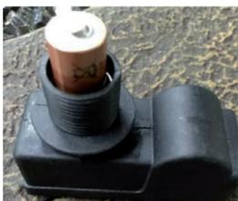
Unscrew the button cap of ignite, put a piece of AAA battery into ignite compartment with anode outward, then screw the button cap (see picture).
