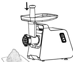
Attach the hopper plate (6) to the top of the filler tube.
