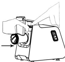
Press the fasten button, hold the head (7) and insert it into the inlet (4) of the motor housing. When inserting it, make sure that the head (7) is slightly tilted (see direction of arrow in figure 1). When you have inserted the head (7), turn it anticlockwise until it is firmly seated (see figure 2).
