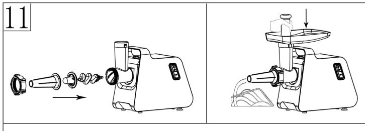
Insert the worm shaft (8) into the head (7) with the plastic end first. Insert the separator into the head (7). Attach the sausage attachment to the head and screw the attachment ring (13) to the head. Make sure that the notches of the separator fits onto the elevations of the head (7).
