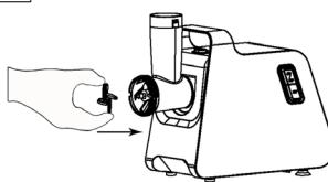
Insert the worm shaft (8), long end first, into the head (7). Turn the worm shaft (8) slightly until it is seated in the motor housing (see figure 3). Place the cutting blade (9) on the worm shaft as shown, with the blade facing forward (see figure 4). If the cutting blade is not fitted correctly, the meat will not be grinded.
