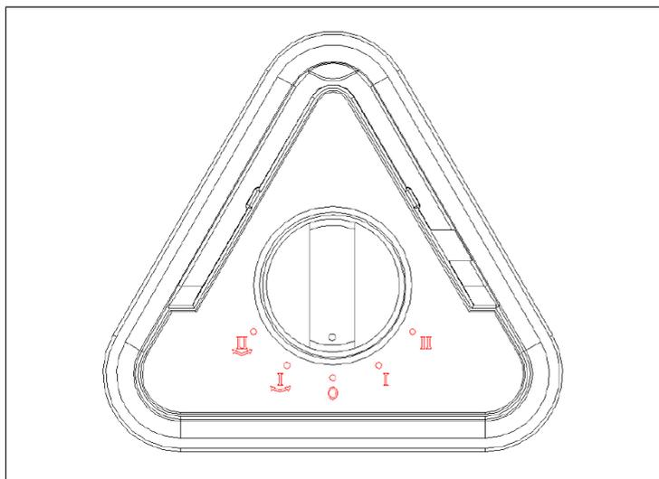
Use the control knob on the top of the unit to set the heating level and oscillation function.
