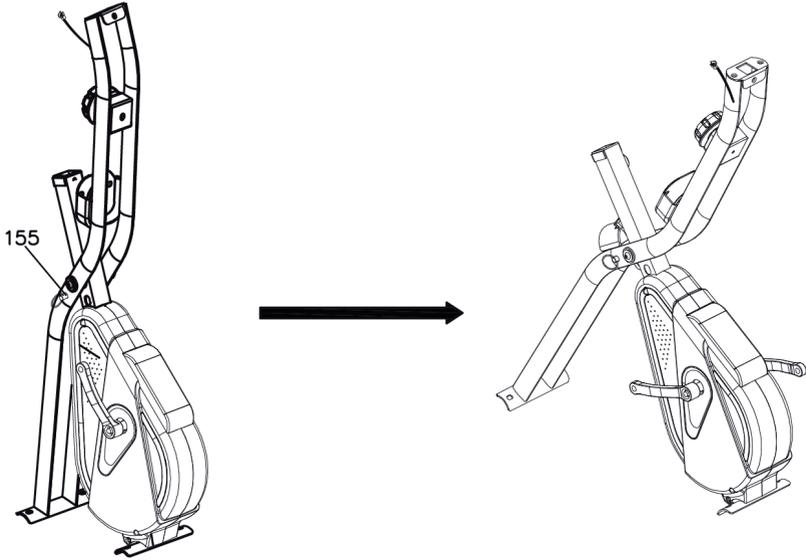
Pull out the pin (155) and unfold the main frame. Then insert pin (155) on the hole of Main frame.
