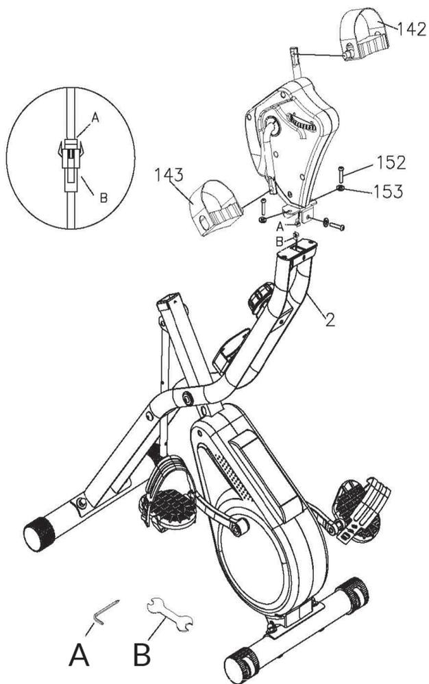
Connect sensor plug A with sensor plug B.
