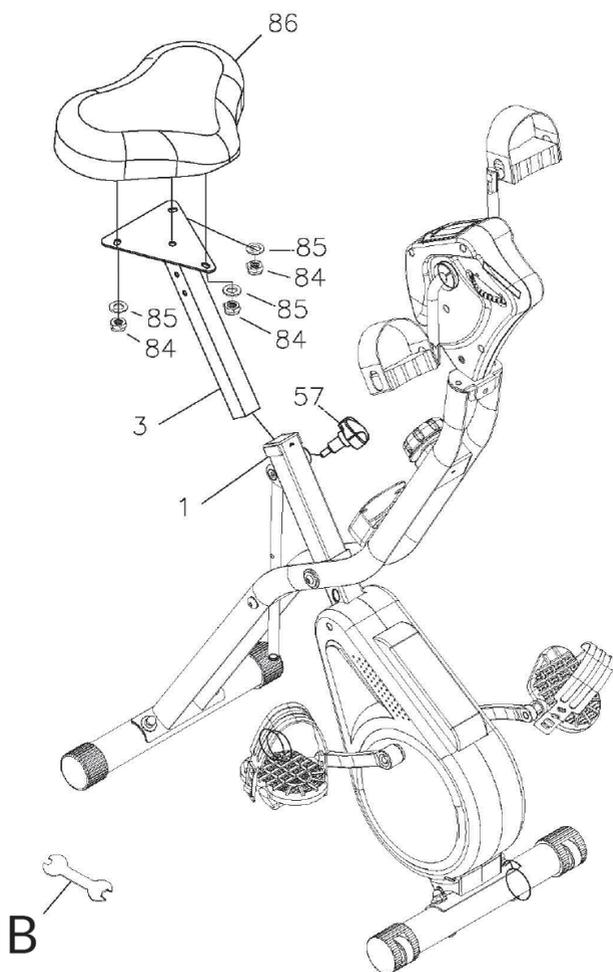
Secure the seat (86) to the seat post (3) with 3 washers (85) and 3 nuts (84).
