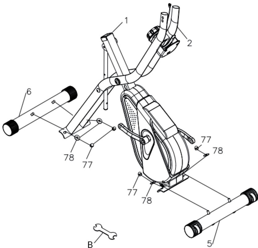
Attach the front anti-roll bar (5) to the main frame (1) with 2 washers (78) and 2 cap nuts (77). Use the tool (B) for this.
