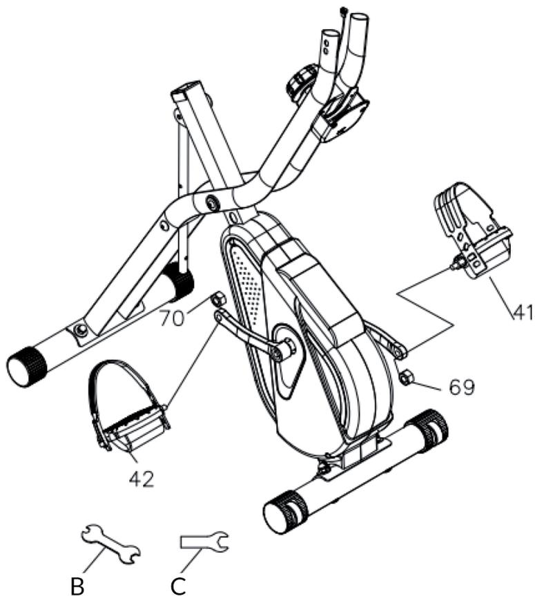
Connect the left pedal (41) to the left crank arm and tighten it with tool (B) while tightening the nut (69) with tool (C).
