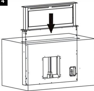
Insert the ventilation system into the cutout and connect it via the retaining rails to the underside of the worktop and the cabinet.
