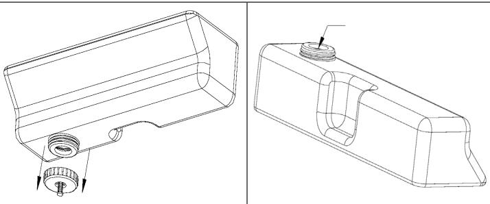
Now turn the stopper on the underside of the water tank and remove it. You can now fill the water tank with fresh water. Then twist the water tank plug back on and make sure that it is properly sealed.
