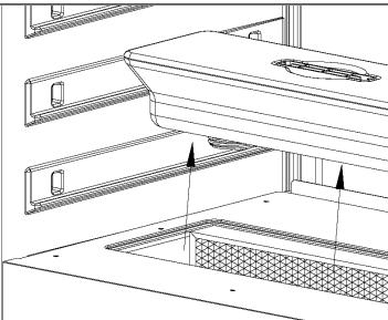
After you have removed the water tank cover, the water tank will become visible. Now remove the water tank from the device in the direction of the arrow.
