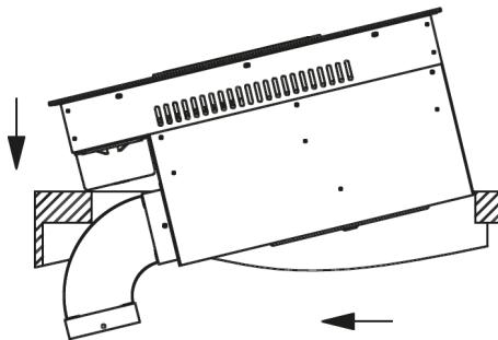
Lift the hob at an angle and slide it into the housing.
