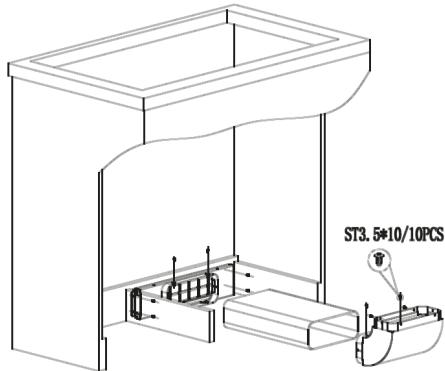
Attach the carbon filter, the plastic tube and the support plate.
