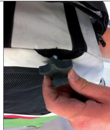
If the trailer frame is lying flat, lift the side walls so that they are vertical. Position the roll bar so that the holes in the side walls and the holes in the ends of the roll bar are aligned (1). Insert the button from the outside on the side wall and then into the thread at the end of the roll bar. Repeat for the other side and tighten both buttons (2).
