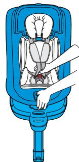
Open the harness buckle position the shoulder straps at the sides of the seat to keep the harness open while position the child.
