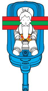
Please note a correctly adjust headrest ensures optimal protection for your child in the safety seat; the headrest must be adjusted so that the shoulder straps are at the same level as your child's shoulders or slightly above. The shoulder straps must run at shoulder height or a little above the height of the child's shoulders.
