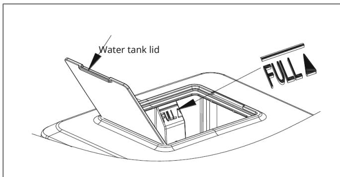
**Note:** Never pour water into the internal water tank, which is located below the ice basket. This water tank is not big enough. Non-observance can negatively affect the ice-making process.
