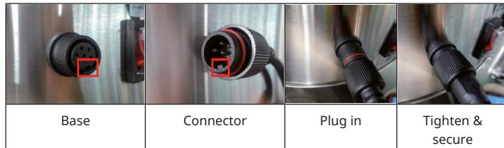
**Note:** Do not overtighten the plug, otherwise the base may come loose or be damaged.
