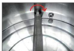
**Einbau des Lochblechs**
