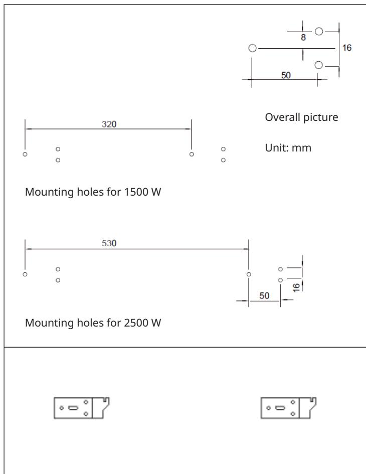
1. Attach 2 brackets to the bottom of the unit (see picture below)
