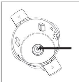
To do this, take the drive coupler and make sure the rubber grommet is in place over the bottom of the coupler as shown below. If you do not attach the rubber seal, liquids may leak from the bottom of the blender jug.
