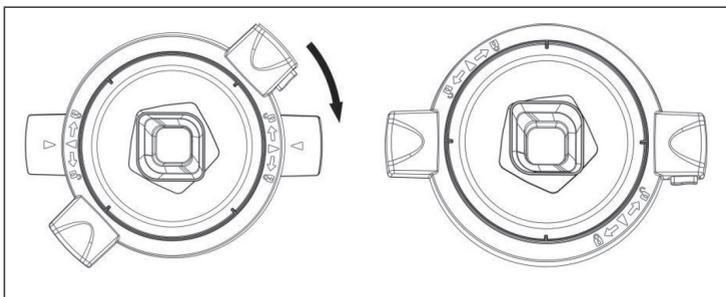
To remove the lid, press the release button, rotate the lid anti-clockwise, and then pull straight up to remove.
