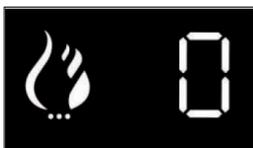
The heating power is displayed in steps from 0 to 10. 10 is the highest setting and means the device heats up faster.
