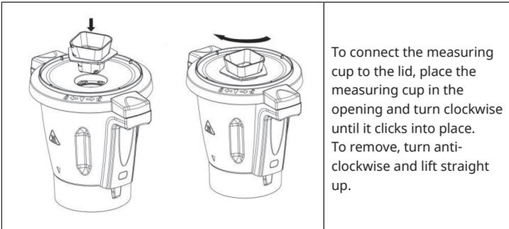
To connect the measuring cup to the lid, place the measuring cup in the opening and turn clockwise until it clicks into place. To remove, turn anti-clockwise and lift straight up.
