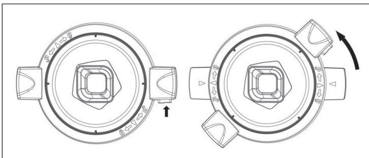
Place the blender jar in the correct orientation on the base unit.
