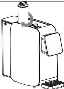
Assemble the new filter element and rotate it clockwise to lighten it.
