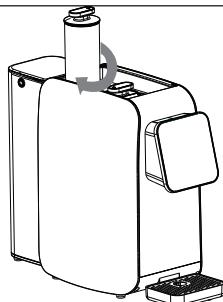
Assemble the new filter element and rotate it clockwise to tighten it.
