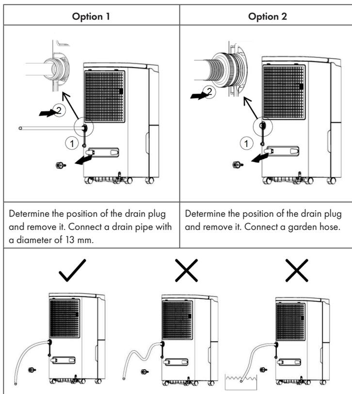
**Note:** The drain line should not be too long (a length of less than 60 cm is recommended). The end of the drain line should be in a lower position than the water outlet (at least 10 cm lower), otherwise there is a risk of leakage.
