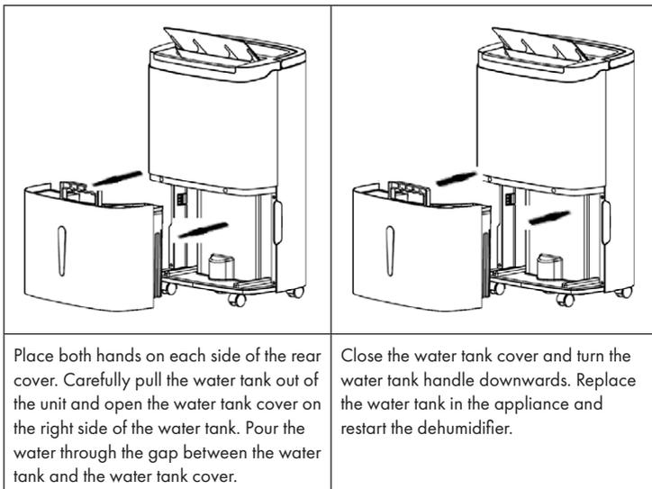
**Note:** Empty the water tank when it is full. Before reinserting the water tank into the unit, make sure that the float is movable or not.
