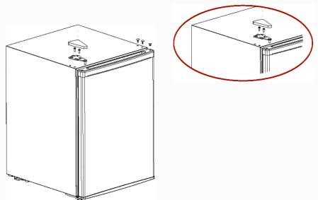
Put the door on lower hinge vertically, and validate the gas tightness of door gasket, then install the upper hinge by fitting screws and the hinge cover, finally cover the hole caps on upper right side.
