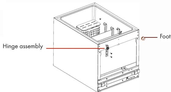
Install the lower hinge and leveling foot on lower left side of cabinet and lower right side respectively.
