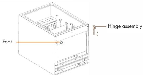
Dismantle the lower hinge assembly and leveling foot.
