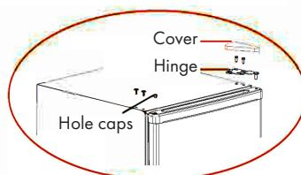
Dismantle hole caps, the upper hinge cover, fitting screws of upper hinge, and remove the upper hinge, please keep the door vertical in whole process for avoiding falling down.
