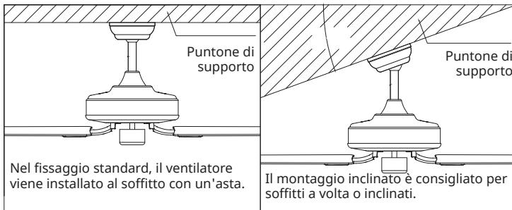
**Fissaggio del supporto a soffitto**
