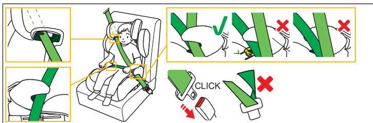
**CAUTION!** Any slack and twist of vehicle belt is not allowed during installation.
