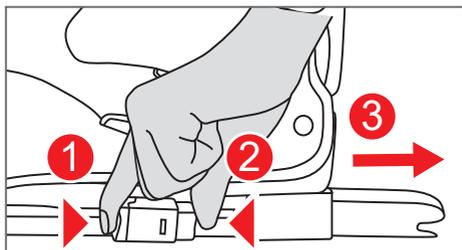
2. Insert both ISOFIX connectors into ISOFIX anchorage points until you hear clear "click" and ISOFIX connector indicator shows green. Then push child car seat to fit vehicle backrest tightly.
