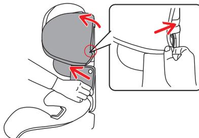
Remove the seat base cover: Remove the cup holder. Then pull the cover from bottom to top to remove it.
