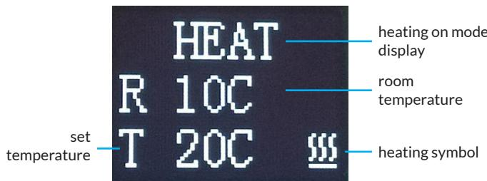
**Heating normally open mode** Short press the ON/OFF button to turn the device on and enter the normal heating mode.
