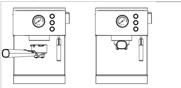
4. Ensure that the steam knob is in the OFF position. Place a cup on the drip tray plate.
