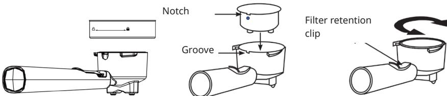
3. Place one hand on the top of the espresso machine to support it and attach the filter holder with the filter holder handle by holding the handle and inserting it into the coffee machine as shown below, then turn it clockwise to the locking position as shown below.
