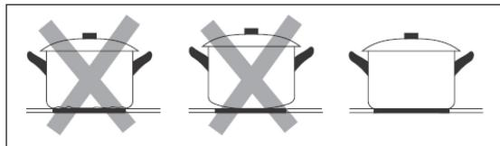
Make sure that the base of your pan is smooth, sits flat against the glass, and is the same size as the cooking zone. Use pans whose diameter is as large as the graphic of the zone selected. Using a pot a slightly wider energy will be used at its maximum efficiency. If you use smaller pot efficiency could be less than expected. Pot less than 140 mm could be undetected by the hob. Always centre your pan on the cooking zone.
