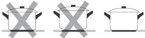
Cookware made of the following materials is not suitable: pure stainless steel, aluminium or copper without magnetic underside, glass, wood, porcelain, ceramics and pottery. Do not use cookware that has sharp edges or a rounded bottom.
