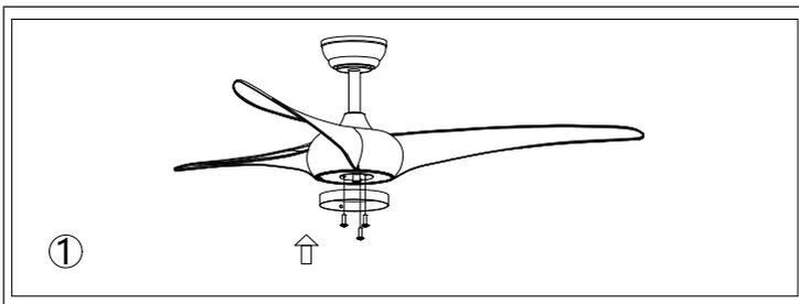
Remove the three screws from the motor connection plate. Carefully tidy up all the wires inside the connection plate. Assemble and align the holes on the back of the LED light with the three screws on the motor connection plate, please see the picture (Fig.1), then tighten the three screws from the hole on the LED plate. Please make sure that the light kit can't be moved after screwing.
