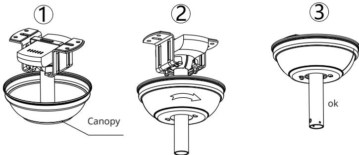
Lift the canopy up to the hanger bracket, aligning the loosened screws in the hanger bracket with the slotted holes in the canopy. Turn canopy to lock. Re-insert screws and secure all screws with screwdriver.
