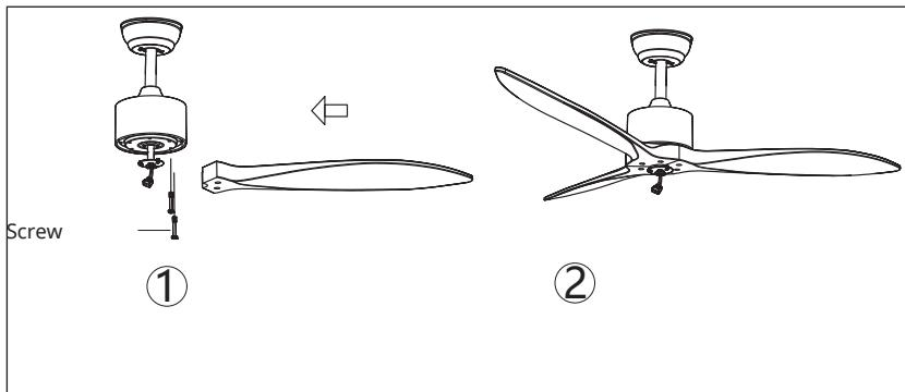
**Time saving:** Washers for blade screws can be fitted to each blade screw before the blades are fitted.
