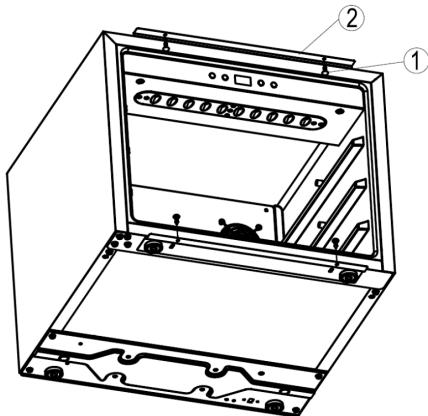
The appliance is equipped with a pair of brackets at the top (②) and at the bottom. This pair of brackets might not be needed and can be removed as per your actual installation situation when you build the appliance into your closet.
