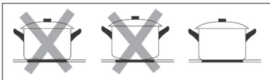
Make sure that the base of your pan is smooth, sits flat against the glass, and is the same size as the cooking zone. Use pans whose diameter is as large as the graphic of the zone selected. Using a pot a slightly wider energy will be used at its maximum efficiency. If you use smaller pot efficiency could be less than expected. Pot less than 140 mm could be undetected by the hob. Always centre your pan on the cooking zone.
