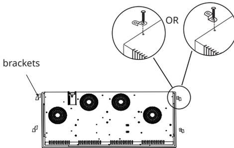
After installation, secure the hob to the worktop by screwing the 4 brackets to the underside of the hob (see illustration).
