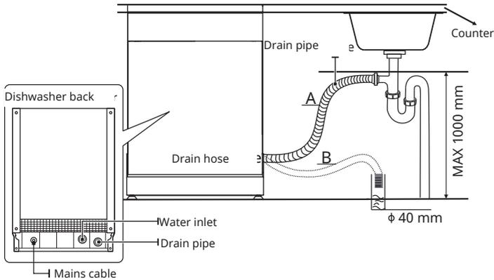
**Note:** Please securely fix the drain hose in either position A or position B
