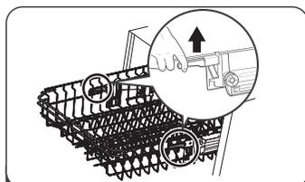
2 lower the upper basket, lift the adjuster handles on each side to release the basket and lower it to the lower position.
