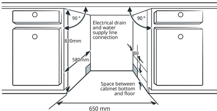
2. If the dishwasher is placed in the corner of the cupboard, there should be some space when the door is opened.
