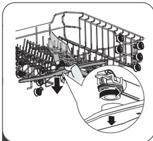
1 To remove the upper spray arm, hold the nut in the middle and turn the spray arm anticlockwise to remove it.
