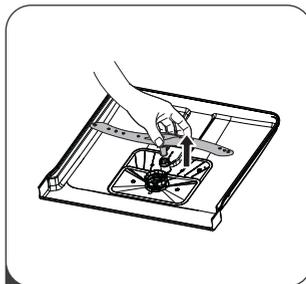
2 To remove the lower spray arm, pull the spray arm upwards.
