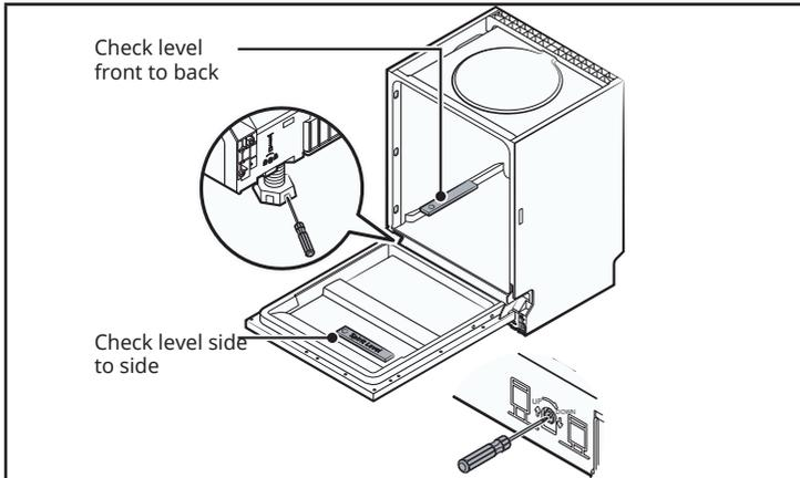
**Note:** The maximum adjustment height of the feet is 50 mm.
