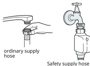
**Note:** If the unit is to be connected to the drinking water supply, it must be fitted with a safety device to prevent the drinking water from being contaminated by backflow (in accordance with DIN EN 1717). We recommend that installation, including water and electrical connections, and repairs are carried out by a qualified technician.
