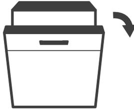
**Note:** The dishwasher door must not be blocked when the automatic door opening is set, as this could disrupt the door lock functionality.
