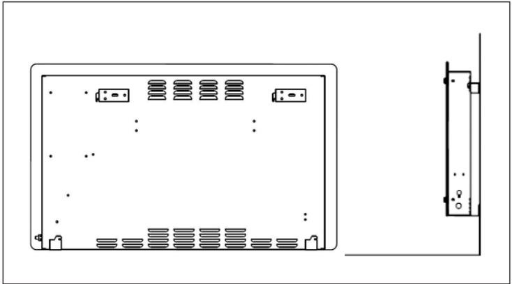
**Note:** To avoid damage, make sure that there are no cables or pipes in the wall before drilling. Make sure that the screws are tight and secure in the wall to ensure a safe wall installation of the heater. Please observe the safety distance given below.
