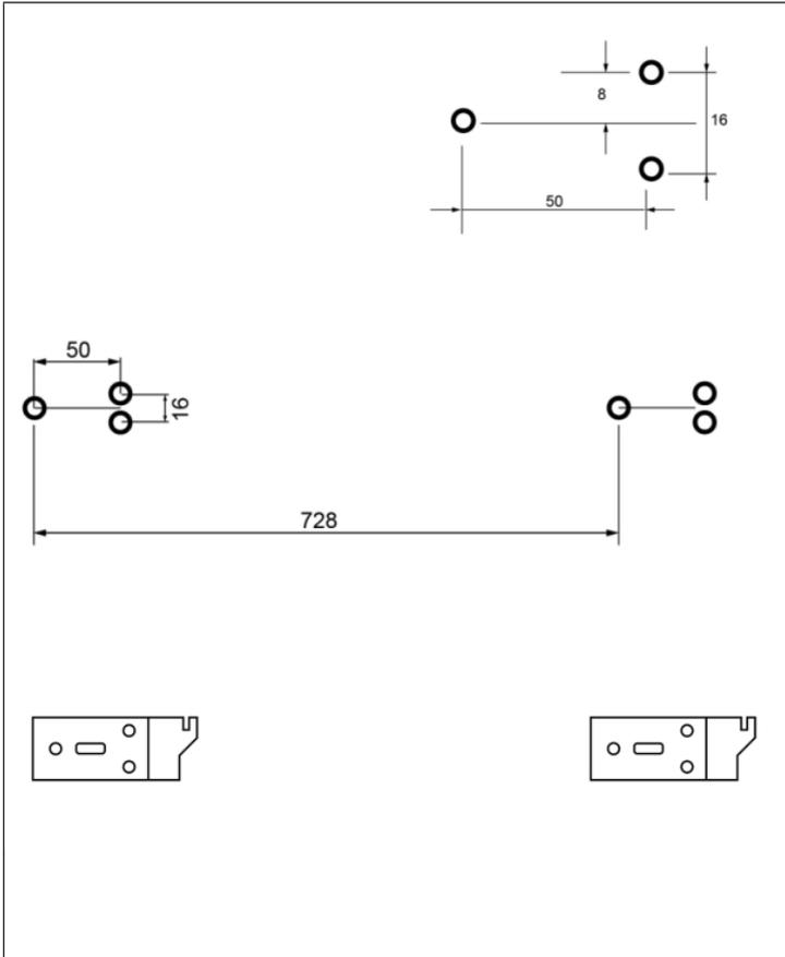
2. Attach 2 brackets to the bottom of the unit (see picture below).
