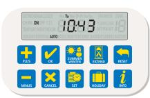
Symbols are used to indicate light level demand, presence sensing and time clock status, combined with clear ON/OFF displays to show the system status for each zone, and temperature sensor if fitted.
