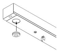
Remember to securely fit grommet strip or a grommet to the hole or channel.
