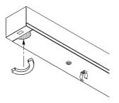
If a circular hole needs to be drilled through the cover plate, for example due to the construction of the fitting, or in the middle of a 6' or 8' fitting (where lamp holders will be wired centrally in the fitting to enable 2 shorter lamps to be fitted end to end), ensure that the hole is large enough for the lamp holder to pass through so that the plate can still be removed in the future for servicing.
