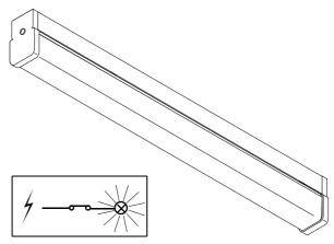
Once completed, a label is to be attached to the outside of the modified fitting. The label needs to be marked using a permanent marker to identify the installer, the date the work was completed. The quantity of lamps within the fitting and the lamp rating should be identified by ticking the appropriate boxes on the label.
