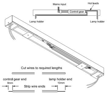
Cut 3mm diameter sleeve to required length to protect wire run through holes and slide onto wire.
