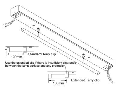
In some cases, additional spacers and longer screws may need to be sourced by the installer where clearances are inadequate when using the standard parts. If there is a louver that will be attached, it may be preferable to adjust the position of the clips so that the clips are concealed by the louver when the fitting is reassembled.
