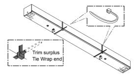
Secure the lamp in to the clips and ensure any exposed cable is left neatly without any strain and clear of any fixings for the diffuser or louver. Remember that some diffuser fixings may need to be attached before inserting the lamp in to the clips.
