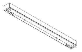
Attach any remaining accessories, ensuring any louvers or diffusers are clean and that any marks applied during the installation are removed from reflectors and lenses.
