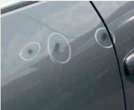
Three dents on one bodywork component
