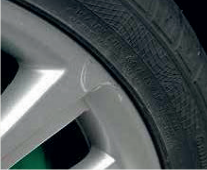
Light scratches on rim flange
