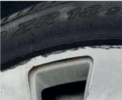
Damage to rim flange with material degradation
