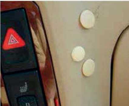
Drill holes in dashboard
