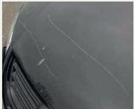
Damage to base coat
