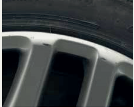
Light scratches without material degradation
