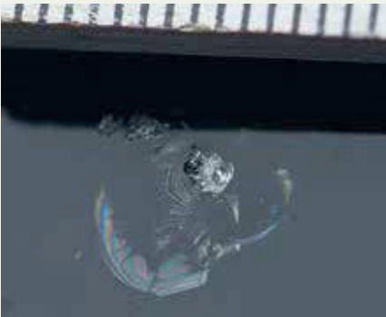
Chip with cracking
