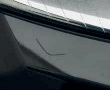
Surface scratches on the paintwork
