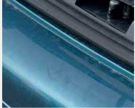
Minor paintwork abrasion
