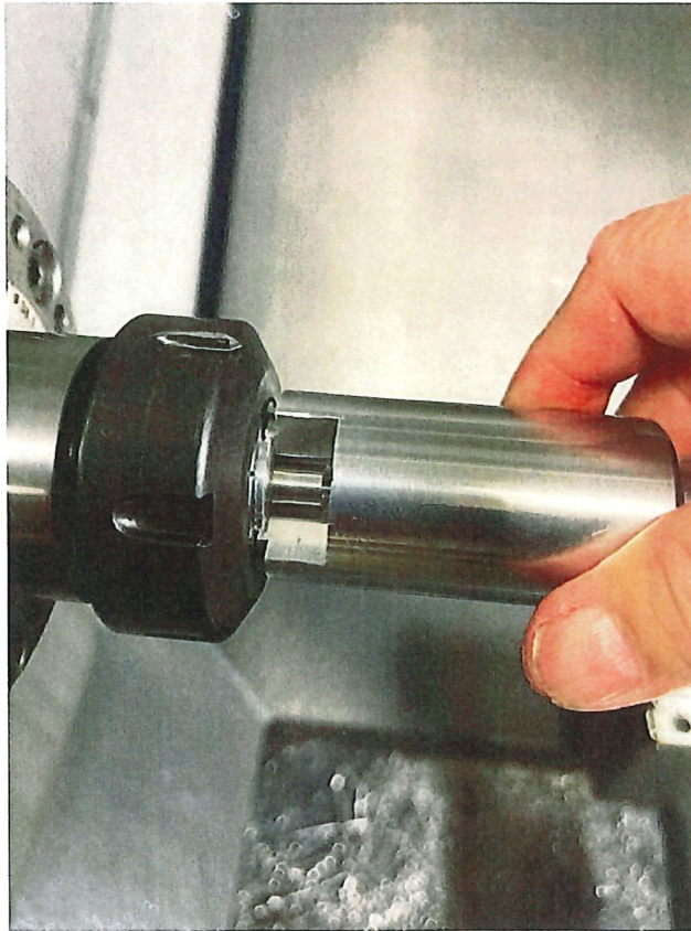
Figure 12 Setting 88L external thread
