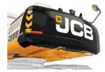
Improved counter weight installation with 6 bolt mounting
