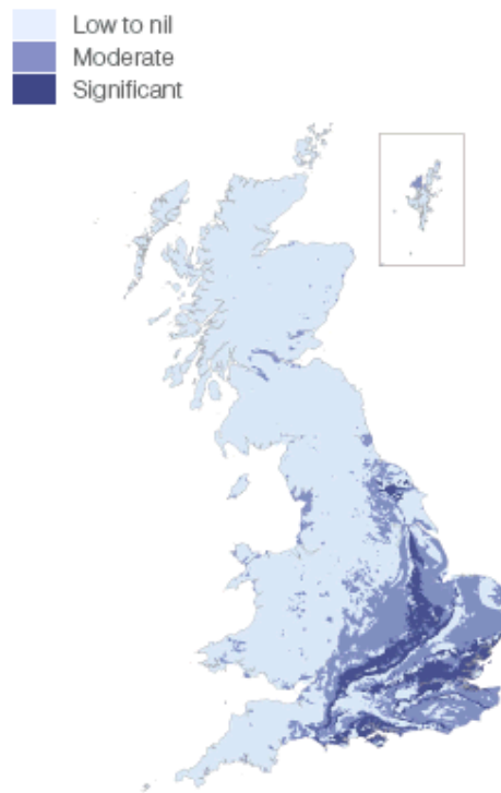
Figure 25: The risk of subsidence due to soil shrinkage (IUK 64 )
