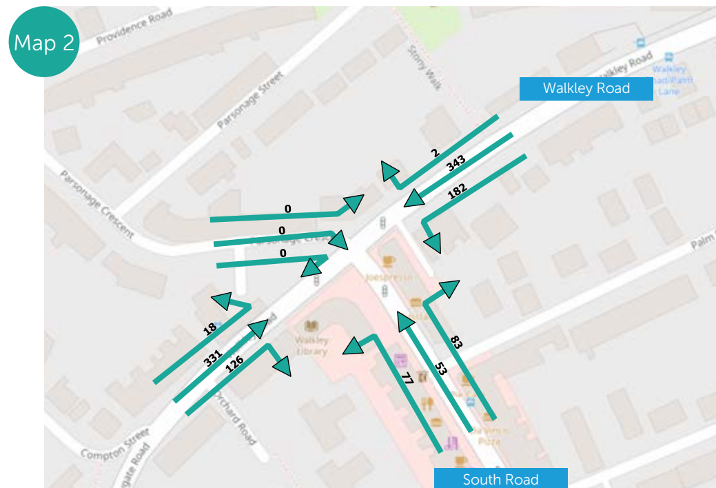
Number of motor vehicles travelling through the Walkley Road / South Road junction in the morning after the scheme (May 2023)
