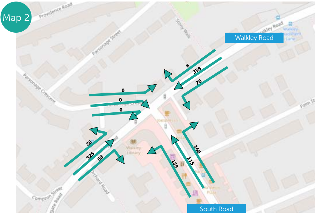
Number of motor vehicles travelling through the Walkley Road / South Road junction in the evening after the scheme (May 2023)
