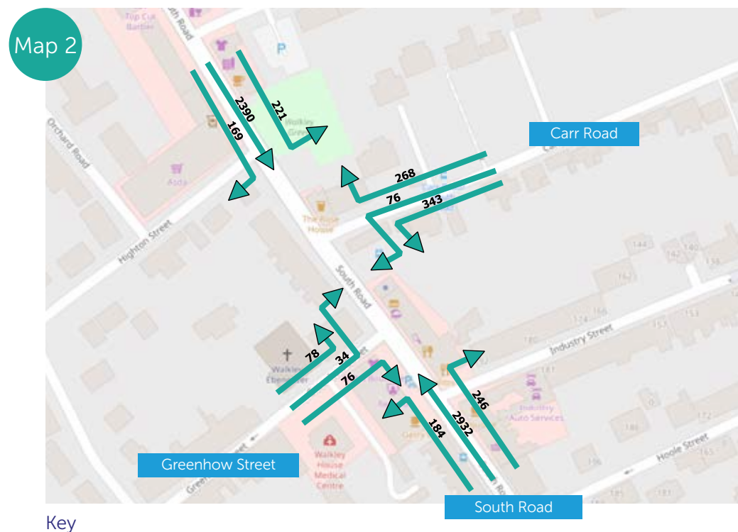
Number of motor vehicles travelling through the the South Road / Greenhow Street junction after the scheme (May 2023)
