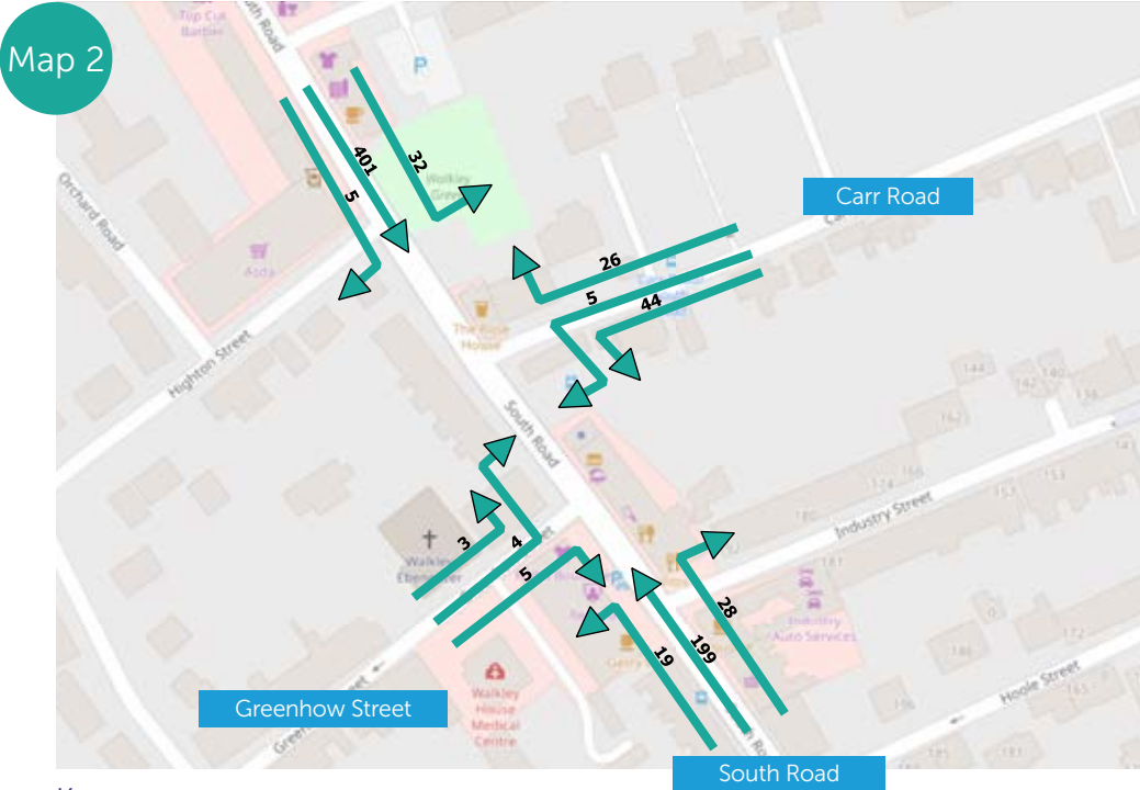
Number of motor vehicles travelling through the South Road / Greenhow Street junction in the mornings after the scheme (May 2023)
