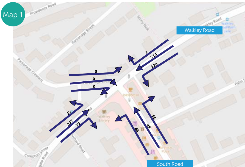
Number of motor vehicles travelling through the Walkley Road / South Road junction in the morning before the scheme (November 2021)
