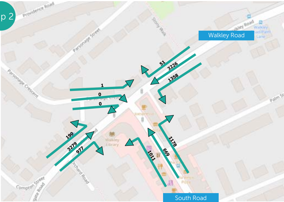
Number of motor vehicles travelling through the Walkley Road / South Road junction after the scheme (May 2023)
