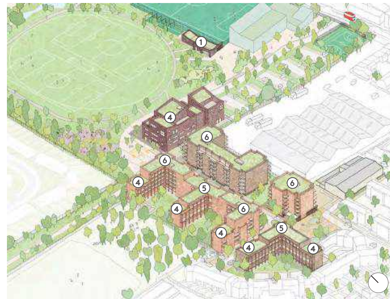
Axonometric view of the proposal illustrating storey heights and stepped massing across the site
