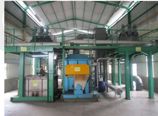
Screw press filter + Sludge Dryer in a Textile Mill
