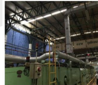
Stenter after installation of recycling system
