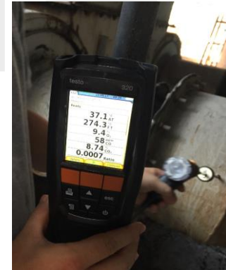
Gas analyser and fuel gas analysis results
