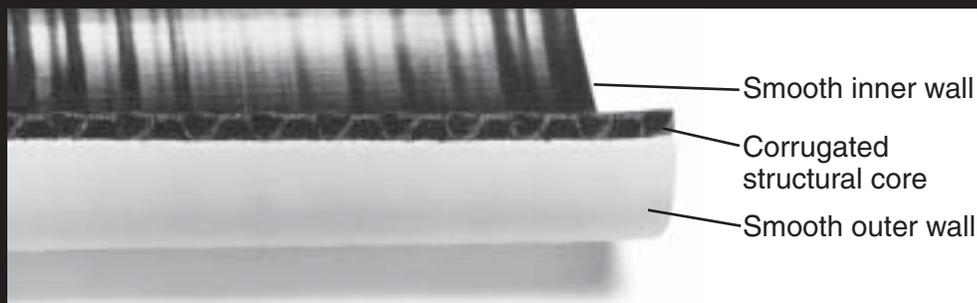
**Three bonded polyethylene layers for exceptional pipe stiffness.** A smooth inner wall is co-extruded with a corrugated structural core, which is then extrusion-laminated with a smooth white outer wall. This construction gives the pipe an unprecedented strength-to-weight ratio, and stiffness ratings at least double that of any competitive sewer and drain pipe.
