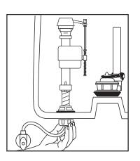
With correct washers in place (see Step 8a), tighten COUPLING NUT 1/4 turn beyond hand tight. DO NOT OVERTIGHTEN.
