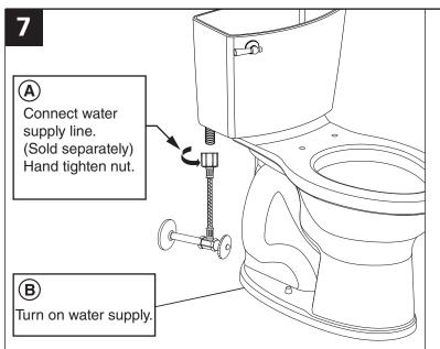
**WARNING:** Overtightening of water supply line nuts could result in breakage and potential flooding. If the connection leaks after hand tightening, replace the supply line. Do not use any type of sealant on the water supply connection. Use of plumber's putty, pipe dope, or any other type of sealant will void the warranty.
