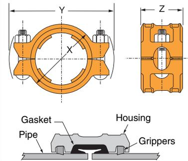
Working pressure and end load are based on a properly assembled Roughneck coupling with bolts fully torqued to the above specifications, on plain-end or beveled standard wall steel pipe and Gruklok Plain- End Fittings.
