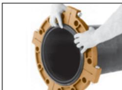
**2** Check the gasket grade to verify that it is properly suited for the intended service. Lubricate the entire surface of the gasket and the flange cavity using the appropriate Gruvlok Lubricant. Place the Gruvlok Flange Gasket around the pipe end by pressing the gasket into the cavity between the pipe O.D. and flange recess. Move around the gasket in both directions until the gasket is fully seated in the flange gasket cavity.
