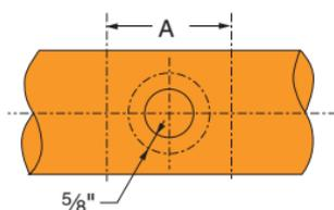
Clamp-T installations require the cutting of a hole through the pipe wall. The hole must be properly sized and located on the centerline of the pipe to assure reliable performance of the Clamp-T gaskets.
