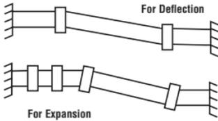
**NOTE: Fully Deflected Joint Will Not Allow For Linear Expansion.**
