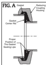
**NOTE:** Fig. A illustrates the correct position of the Fig. 7010 Reducing Coupling gasket and housing properly assembled onto adjacent pipe ends.
