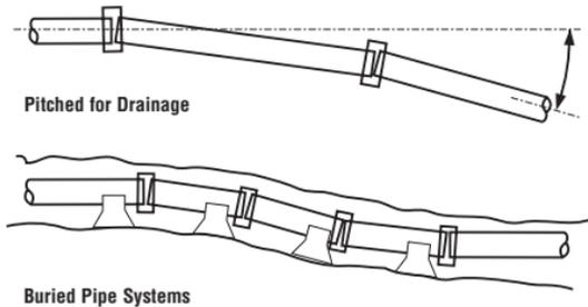
Pitched drainage systems, buried pipe systems where pipe laying conditions are subject to settlement, and exposed pipe systems laid on rough ground are but a few of the many types of pipe installations that present conditions where the functional capability of the Gruvlok coupling are useful.
