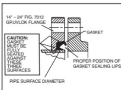
**3** The correct position and relationship of the components of the Gruvlok Flange assembly is shown in the Figure above. The wide gasket lip must seal on the pipe surface diameter and the narrow gasket lip must face the mating flange. Be careful that foreign particles do not adhere to lubricated surfaces.
