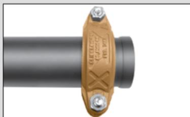
**A.** Slide the coupling on the pipe past the groove. The bolts and nuts can be hand tightened to position the coupling in place.
