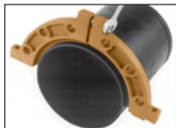
**1** Place each Gruvlok Flange segment around the grooved pipe with the key section fitting into the groove and the flange gasket cavity facing the pipe end. Loosely assemble the segments using the four segment-bolts-and nuts. Alternately and equally tighten the latch bolts and nuts to the specified latch bolt torque. Bring the four flange segments into full, firm metal-to-metal contact.
