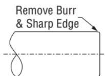
Square cut pipe with O.D. burr & sharp edge removed is preferred configuration.
