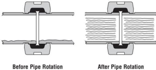
Utilizing the rotational capability of the Gruvlok Coupling, the pipe life of a slurry or similar coarse material piping system can be extended.
