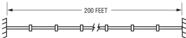
Thermal expansion tables show this system will expand a total of 1.80" due to the temperature change .
