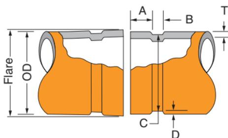
End Guard (EG) roll groove is designed for lightwall pipe to be joined by HPR 7004 EG couplings.
