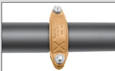
**C.** Slide the coupling back over the grooves so that the coupling keys are located over the respective grooves on both pipe ends.
