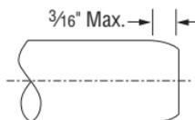
Soft pipe when roll cut may be swaged inward. Swaged portion not to exceed 3/16"
