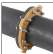
**CAUTION:** Proper torquing of flange bolts is required to obtain specified performance. Over torquing the bolts may result in damage to the bolt and/or casting which could result in pipe joint separation. Under torquing the bolts may result in lower pressure retention capabilities, lower bend load capabilities, joint leakage and pipe joint separation. Pipe joint separation may result in significant property damage and serious injury.
