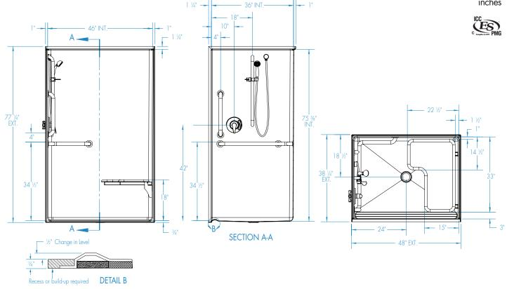
FEATURES Dimensional Tolerance ± 3%". Dimensions needed for site preparation should be measured from the unit. Aquatic assumes no responsibility for preparatory work.
